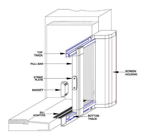
Very often this condition exists on three sided, but must be created at the threshold. In most situations, sill adapters will allow you to create this condition so that the bottom track can be mounted.
